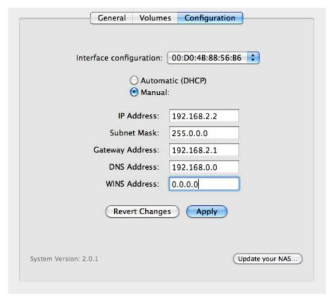
Assign a Static IP compatible with your network
