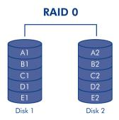
**Caution:** If one physical disk in a RAID 0 array fails, all data will be inaccessible since parts of every single file have been written to both disks.
