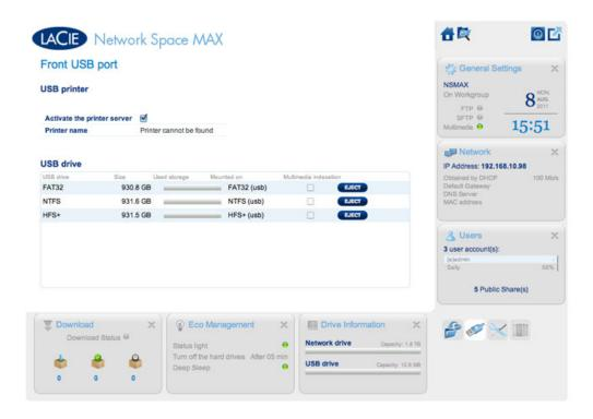
This page provides information on devices connected to the front USB expansion port. Please note that the rear USB device port is meant to plug the network storage device to your computer.
