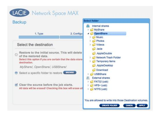
• To free disk space, you can choose to clear the source before the job starts. By checking the box in this step, all data will be erased in the source directory. Before continuing to the next step, a prompt will ask you to acknowledge that all data will be erased in the source before the restore begins.
