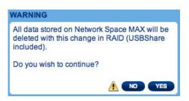
10. Synchronizing to RAID 1 will take four or more hours depending upon the capacity of the hard drives. RAID 0 should not take longer than five minutes. While the network storage will briefly go offline when building the RAID configuration, you will have access to the storage once Synchronizing begins. A green check mark will appear in the RAID status window once the RAID configuration is complete.
